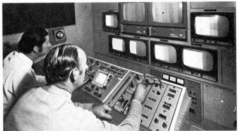
The Harlech colour television outside broadcast vehicle (right) is equipped with four of the EMI colour television cameras type 2001 and is sub-divided to provide separate control areas for production, sound and vision. The sound facilities provide for 24 inputs into six groups. The vision system allows simultaneous mixing and special effects operation from up to ten inputs and a separate caption scanner.
