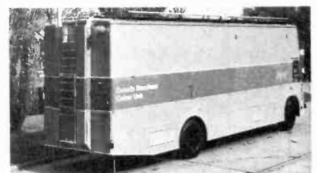
The Harlech colour television outside broadcast vehicle (right) is equipped with four of the EMI colour television cameras type 2001 and is sub-divided to provide separate control areas for production, sound and vision. The sound facilities provide for 24 inputs into six groups. The vision system allows simultaneous mixing and special effects operation from up to ten inputs and a separate caption scanner.
